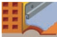
e= 1mm. (filled with mortar)
